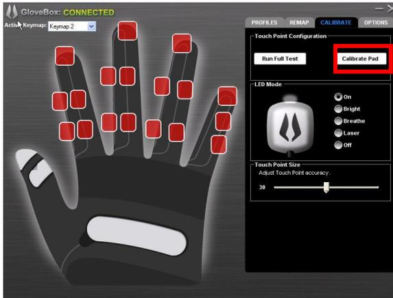
Figure 10. Calibrate Pad Screen
